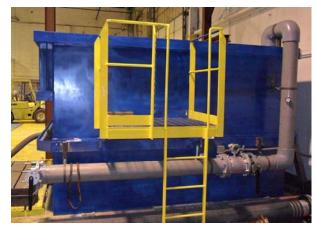
submersible pumps. While other pump rebuilders in the market are limited to static testing, we are now able to actually run most pumps under loaded conditions. We are in a unique position to verify the quality of our repairs, solve customer problems and provide accurate pump performance data."
